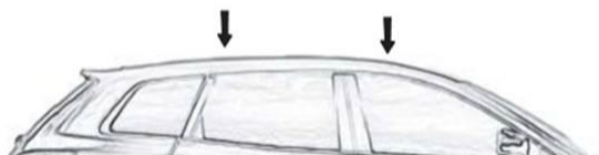
Location of anchor points on vehicle
